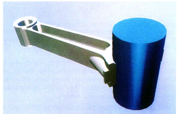
**Figure 1.** A small mechanical assembly: The interference between the cylinder and the connecting rod is not apparent.
