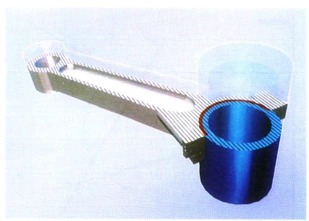
**Figure 9. Interference highlight:** The solid-clipping technique of Figure 4 is enhanced by highlighting (in red) the cross-section regions where pairs of solids interfere. The portion of the assembly removed by the cut-volume is displayed in transparent mode.
