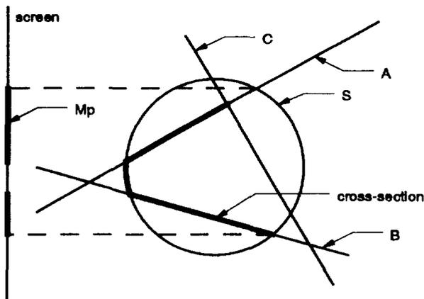
**Figure 7. Masking for a clipping-product:** Two front clipping planes A and B and one back clipping plane C bound a clipping-product. Mp is constructed by scan-converting S clipped by A and B. The visible cross-sections are obtained by rendering A (clipped to B and C) and B (clipped to A and C) over pixels where Mp is 1.
