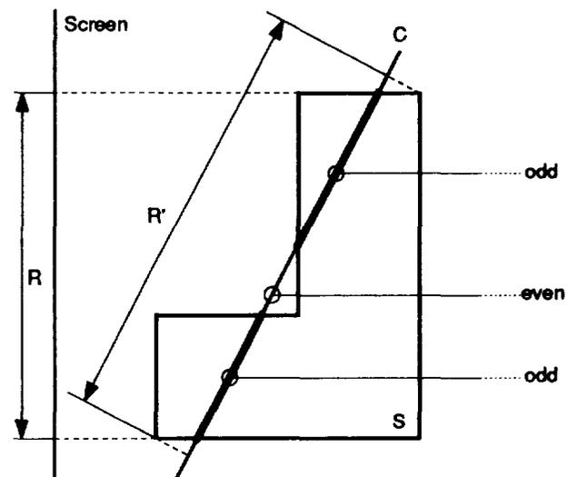
**Figure 5. Parity-based mask construction:** The pixel-mask,  $M_p$ , for the intersection of plane  $C$  with solid  $S$  is computed by toggling the mask during the scan-conversion of the faces of  $S$  behind  $C$ .  $R$  is the projection of  $S$  onto the screen and  $R'$  the projection of  $S$  onto  $C$ .
