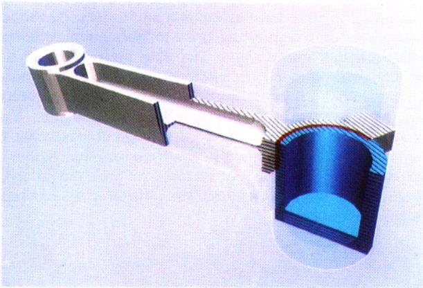
**Figure 2. Graphics inspection techniques:** A multi-facet cut-volume is removed to show the internal structure of the assembly. The resulting cross-sections are displayed in the appropriate color and hatched. Red areas indicate interferences.
