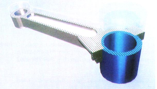
**Figure 4. Solid-clipping:** In addition to the surface clipping of Figure 3, the cross-section of each solid by the clipping plane is hatched and shaded using the color of the solid.
